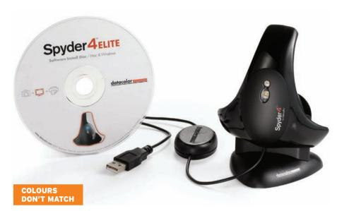
Datacolor Spyder 4. It measures your screen colours and creates a colour profile to match. A similar device is available to calibrate printers; using the two together you should be able to achieve accurate colour reproduction.
