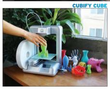
of 0.2mm and can produce objects up to 140x140x140mm in size.
